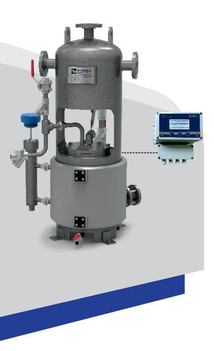
The Forbes Marshall mPump, Miniature Condensate Pump package unit, is a positive displacement pump unit operated by steam, compressed air or pressurised gas. The compact pump has an in-built receiver for condensate, which eliminates theneed for a separate storage tank. The size enables this pump to be used for recovery of condensate from equipment with very small steam loads and where steam consuming equipment is located far away from the process section.
