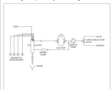
After rinsing the cuvette, sample will pump into dilutor followed by distilled water into the cuvette. Mixing pump will then activated to mix the sample with distilled water (dilution process applies to high range models only. For low range models sample will pump directly into cuvette).
