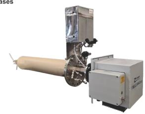
The FMGCEM40xx insitu model is field proven and is the most preferred continuous emission measurement technique in the industry. The insitu measuring probe mounted on the stack / duct has an intrusive stainless steel measurement chamber equipped with sintered diffuser filter which allows flue gases, excluding particulate, to enter into the measurement chamber.
