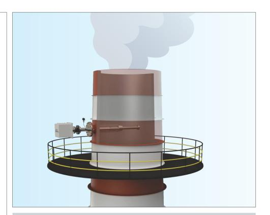
Gas analysers provide useful information about the composition and characteristics of stack gases being emitted. This enables the plant to gain valuable insights on the combustion efficiency, emissions monitoring, safety and troubleshooting.
