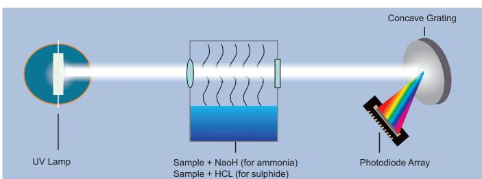
The measuring principle is based on UV light absorption spectrum of ammonia gas NH<sub>3</sub> in equilibrium with dissolved ammoniac gas in the water sample.
