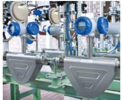
PCT safety equipment with OPTIMASS 6400 fitted in series
