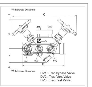
Dimensions / Weight (approx.) in mm and kg (Valves in closed condition)
